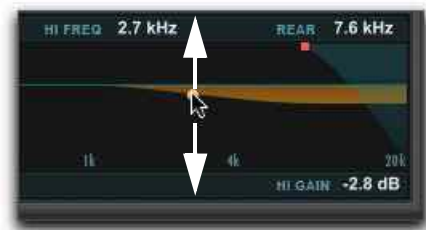
Cutting or boosting an EQ frequency band
